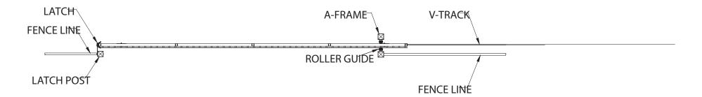
2. SET A-FRAME AND ROLLER GUIDES TO MAKE SURE THE GATE RUNS SMOOTHLY IN OPEN AND CLOSED MOVEMENTS.
